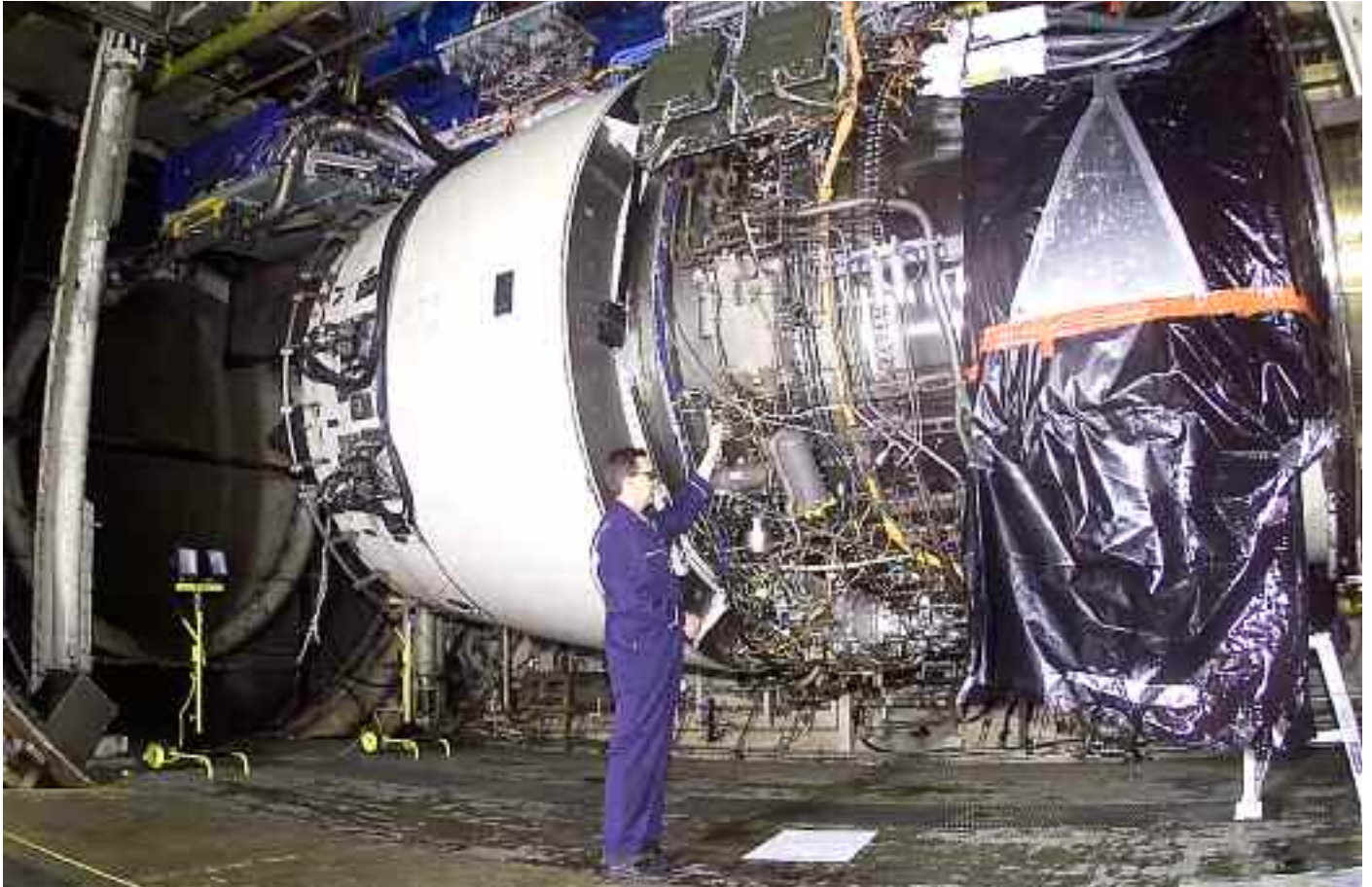
Rolls-Royce fitter checks instrumentation on a Trent 900 engine.
